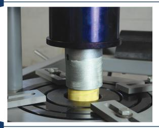
"Jog" the ram by quickly depressing and releasing the "on" button on the remote control switch,
