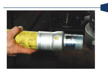
Note: If the gauge reads 10,000 PSI before swaging is complete, stop. The ferrule or die used for that hose end may be incorrect. Contact Dixon<sup>®</sup> for further assistance.
