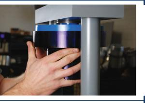
Before you begin, make sure the ram is fully re-tracted, and remove the **25PUSH400** (also referred to as the pusher hat) from the main pusher plate, if installed on the ram.
