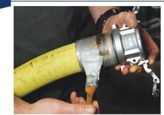
b. Lubricate the outside of the ferrule with Crisco<sup>®</sup> (recommended) or a high viscosity oil or heavy duty grease.
