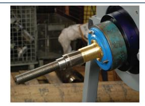
Screw (or slide) the IX plug, small end first, onto the pull rod and into the shank of the stem. For 2" and above screw the retaining nut on until it contacts the plug. Move the stem slightly to allow for slack and hand tighten the plug or nut until it is snug.
