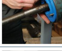
Slide the stem over the pull rod and into the recess of the thrust plate with the connection side of the stem facing the ram. For male stems, insert the hex into the recess of the thrust plate. For female stems, insert the first hex into the thrust plate so that it goes all the way through, so that the second hex will fit into the recess of the thrust plate.
