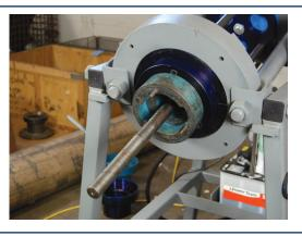
Select the corresponding thrust plate for the size fitting that you are installing. Ensuring that the recess is facing outward towards the operator, slide the thrust plate over the pull rod until it reaches the **25ROSTPA**. Align the holes in the thrust plate over the pins. Tighten the wing nut to lock it in place.
