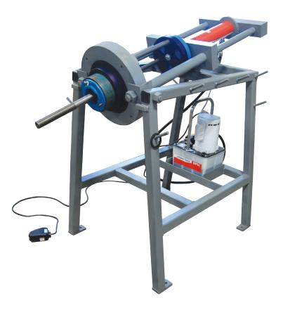
**Dixon** 800 High Street • Chestertown, MD 21620 ph: 877•963•4966 fax: 800•283•4966 *dixonvalve.com*  Before you begin, make sure the Ram is fully retracted. Install the Holedall Petroleum Thrust Plate Adapter (**25ROSTPA**) to the end of the **25IXATTACH** with set screws. Select the proper Pull Rod.
